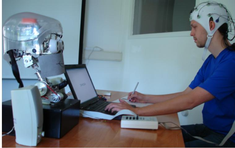
**Fig. 1.** Picture of the recording setup with the robot to the left, the computer for the secondary task in the center and a participant wearing an EEG cap to the right.
